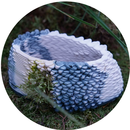
3D printed gradient ceramic with textures and probiotic bacteria enhancing the moss growth
