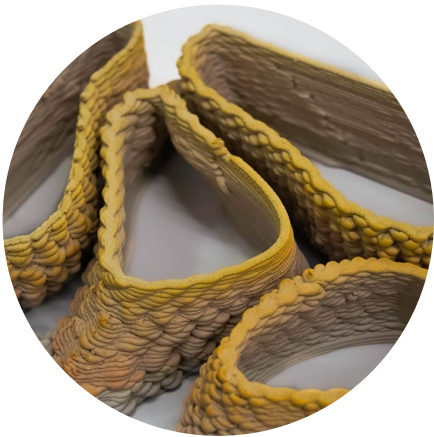
Multimatierial deposition tool computational workflow were specifically designed to achieve gradient robotic 3d printing
