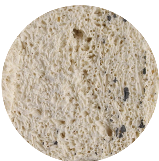
Highly porous ceramic different porosities for water retention
